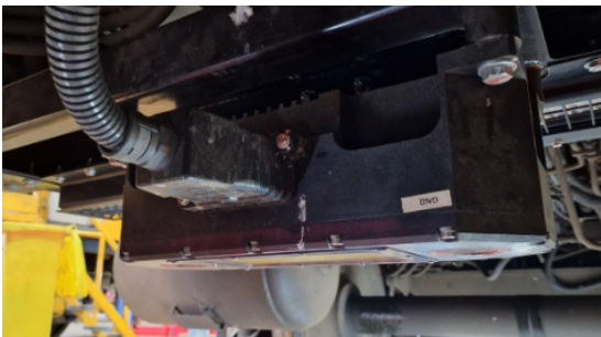
Figure 1 - RailLoc installed on a Class 153
